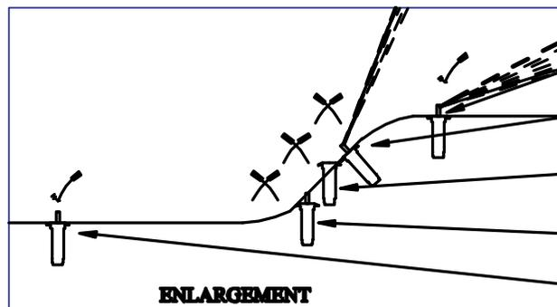
**PREFERRED SPRINKLER LOCATION - VERTICAL ALIGNMENT OF SPRINKLER - PROVIDES EVEN WATERING OF TEE (UNIFORM IRRIGATION)**
